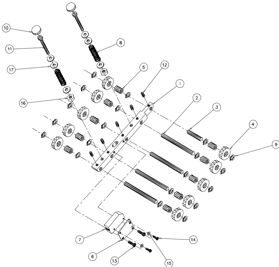
**INTERMEDIATE DRIVE PULLEY ASSEMBLY (Fig. 6-15)**
