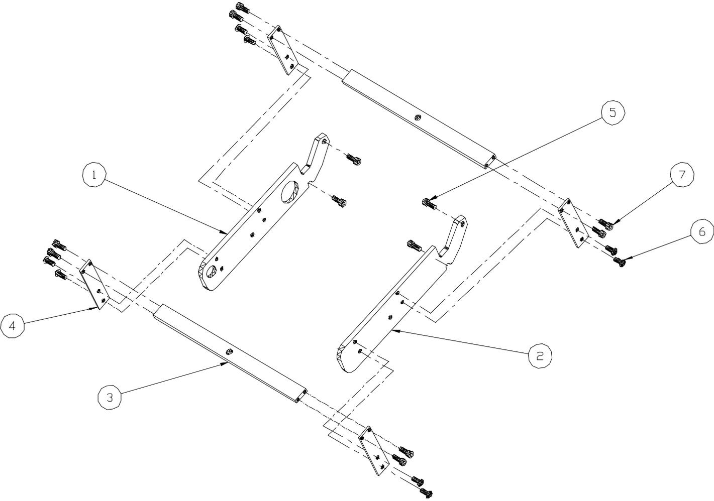
**ACCELERATOR SHAFTS ASSEMBLY (fig. 6-13)**
